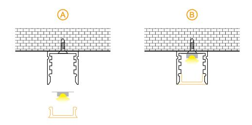
**NOTE**: Fixing screws must be fully recessed and provide flat surface for LED
