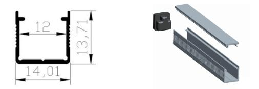
The 1414 is designed to fit inside standard stainless steel tube with a 15x15mm slot which enables the supply of LED handrail as componentry only.
